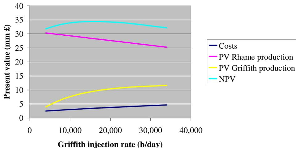
It is useful to note that for the larger field, Rhame, it probably suffices to make three reservoir simulation runs. Since the percentage changes in water injection in Rhame are relatively small, the effect of the changes is likely to be approximately linear. If this is the case, then all one needs do is run the Rhame reservoir simulation model with
