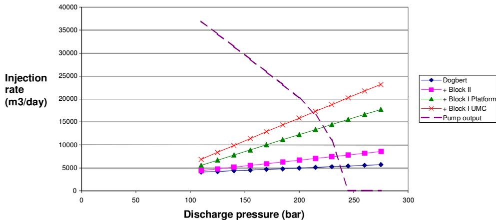
From the gradient of the Dogbert injection rate vs pump discharge pressure curve, one can calculate how much the discharge pressure has to be increased to inject an extra 1 m<sup>3</sup>/day into Dogbert - 0.1 bar, as it turns out.
