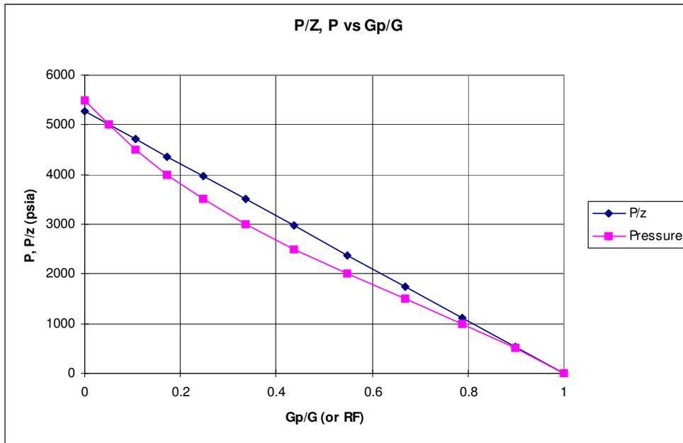
The P/z plot is a straight line between  $P_i/z_i$  and  $G_p/G=1$ .
