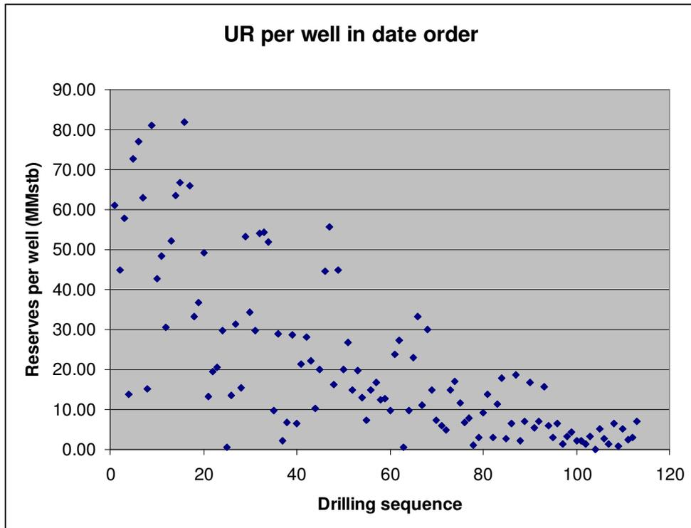
The diagram below shows the recovery per well for all producers drilled into the field since between 1992 and 2001. In order to ensure that the results do not penalise the wells drilled last, each well's ultimate recovery has been predicted from decline curve analysis on each well. In other words the recovery per well is the forecast UR over its lifetime, not cumulative production to 2001.
