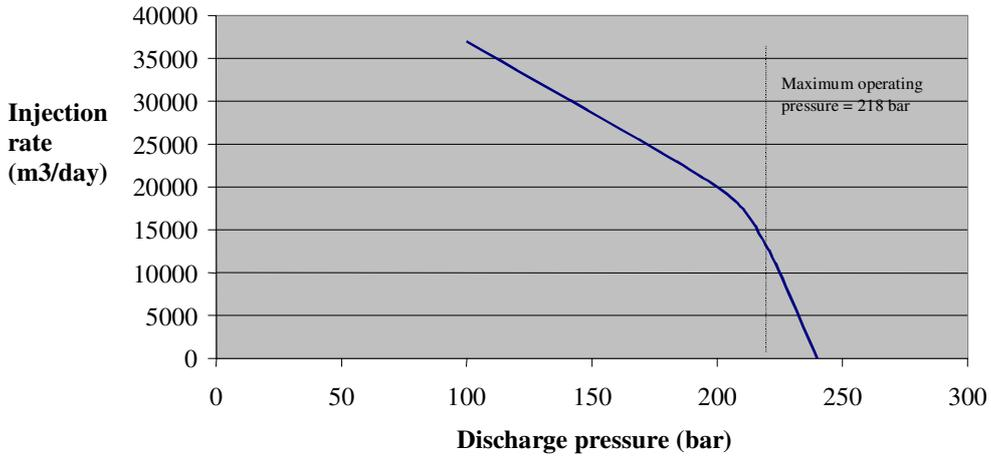
It is clear from the pump PQ relationship that if you start with all the wells open and then gradually shut Block I injectors, you will increase the HP discharge pressure and reduce the overall flow-rate from the pump. If, then, the overall flow-rate is being reduced, it is clearly not correct to assume that
