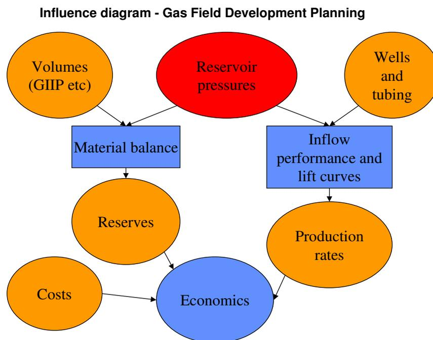
In many respects, reservoir pressure is the key parameter, since it links the material balance and the calculations of production rates.
