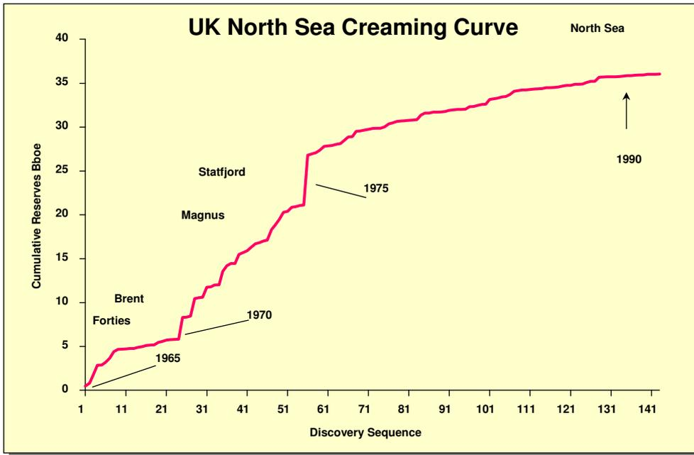
In an infill drilling situation, an equivalent of the creaming curve can be used to predict the performance of sequential infill drilling targets, and this can be based on the well performance to date.
