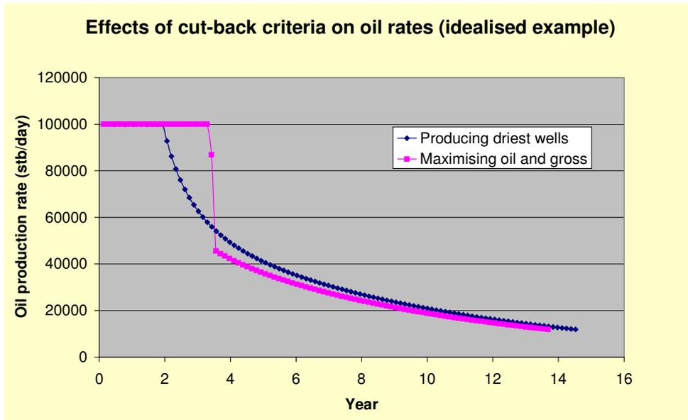
NB - For the strategy of maximising both oil and liquid, there is a sudden drop in oil production. This is an artificial feature that is the result of the artificial assumption made in constructing this extreme case – the assumption that maximum oil and liquid rates can be maintained up to
