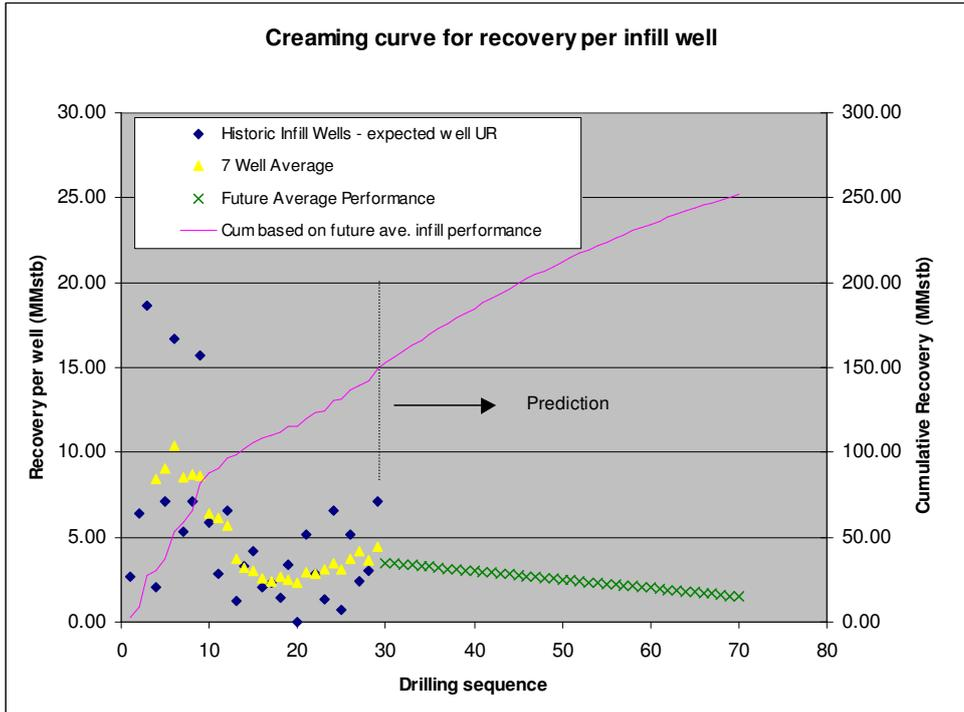
The above plot shows the cleaned up data set, comprising only true infill producers drilled since 1992. The creaming curve is used to predict the future infill well performance, providing an estimated remaining reserve of 100 MMstb from infill drilling. The well performance ranges from 3.5 MMstb for the first infill well, down to 1.5 MMstb for the fortieth infill location. This performance can be used to create an infill production profile.
