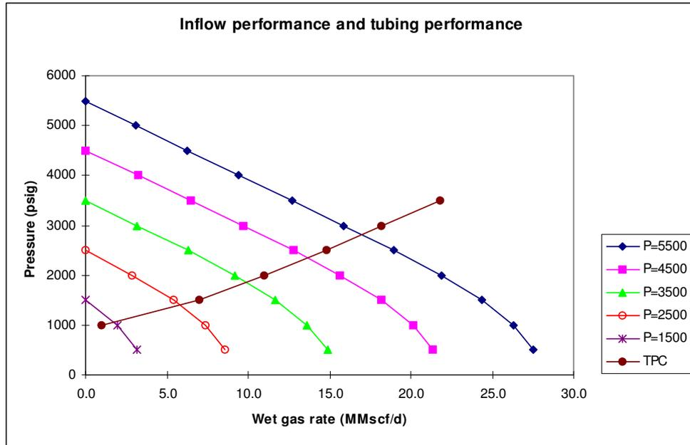
This plot will be used to determine well productivity for any current reservoir pressure.
