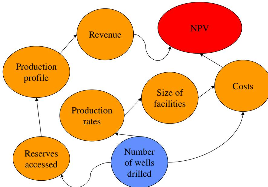
The first effect of increasing the number of wells in a field development plan is to increase costs. Assuming that the facilities are scaled to the number of wells, both opex and capex are likely to be approximately a linear function of the number of wells in the plan. In consequence, the present value of the total costs will also be approximately a linear function of the number of wells, of the form  $a + b.N$ , where
