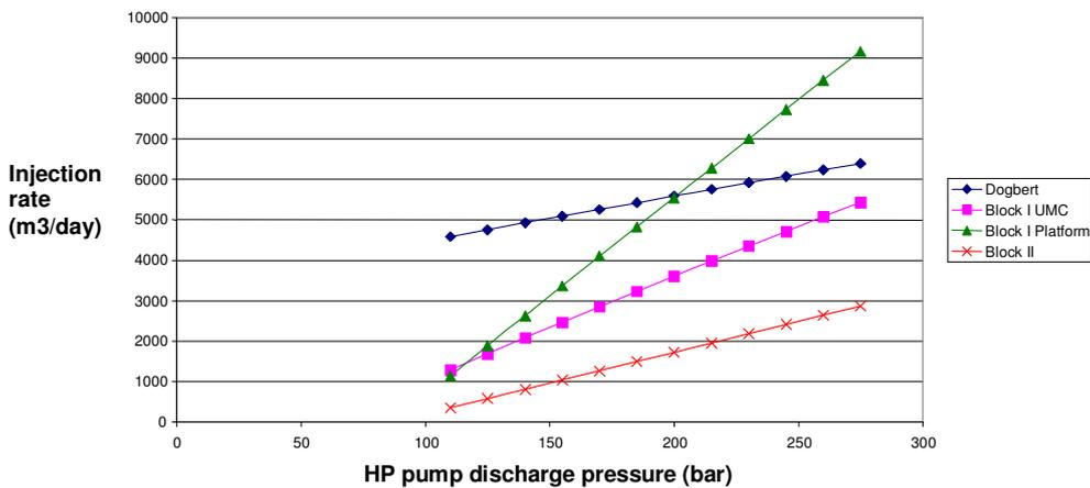
When the combined flow-rate into all the open injection routes (i.e. what the fields can take) is plotted together with the HP pumps' P-Q curve (i.e. what the pumps can deliver), the intersection of the two curves gives the flow-rate that would occur for that combination of open injection routes.
