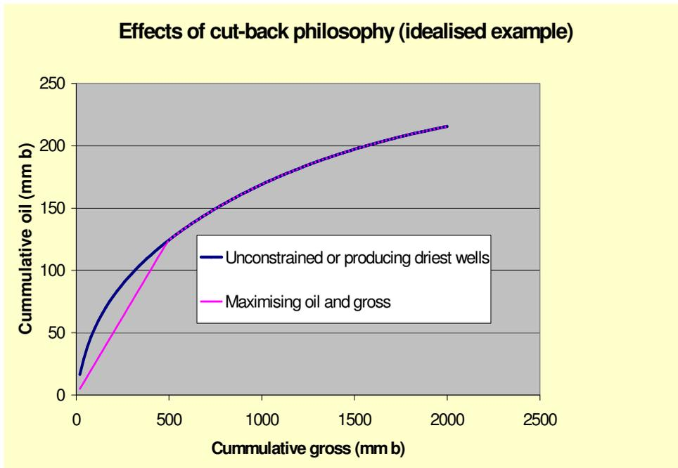
A cut-back strategy of producing the driest wells will lead to all the wells having similar water-cuts (if some are drier, they are produced preferentially until their water-cuts build up. Hence, if the wells are similar, the cumulative oil vs cumulative gross relationship with a driest wells cut-back strategy is very similar to the unconstrained relationship.
